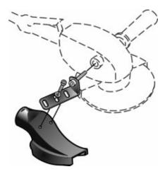
The adapter can hold the nozzle in two positions to match Ø180mm (7") or Ø230 mm (9") grinding wheels.
