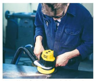
180 mm kit (7") fitted to heavy metal grinder. Turning the snap-in hood compensates for a decreasing grinding disc diameter.
