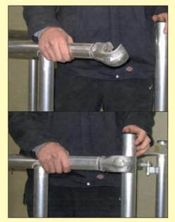
With the platform in place the gate can be unclipped from its parking position and locked on to the vertical of the frame.
